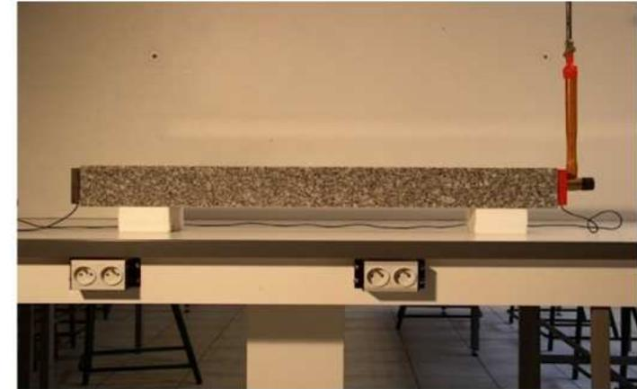
Experiment set-up: the two piezoelectric cells are connected to the sound card of the computer. The shock must be strong enough to clearly visualize the wavefront. Measurements can be made with 1m to 1.5m bars (steel, granite, wood, polystyrene ...)
